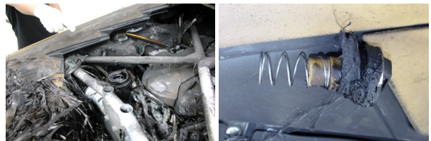
Photo. 8 Water reserver tank stopper
