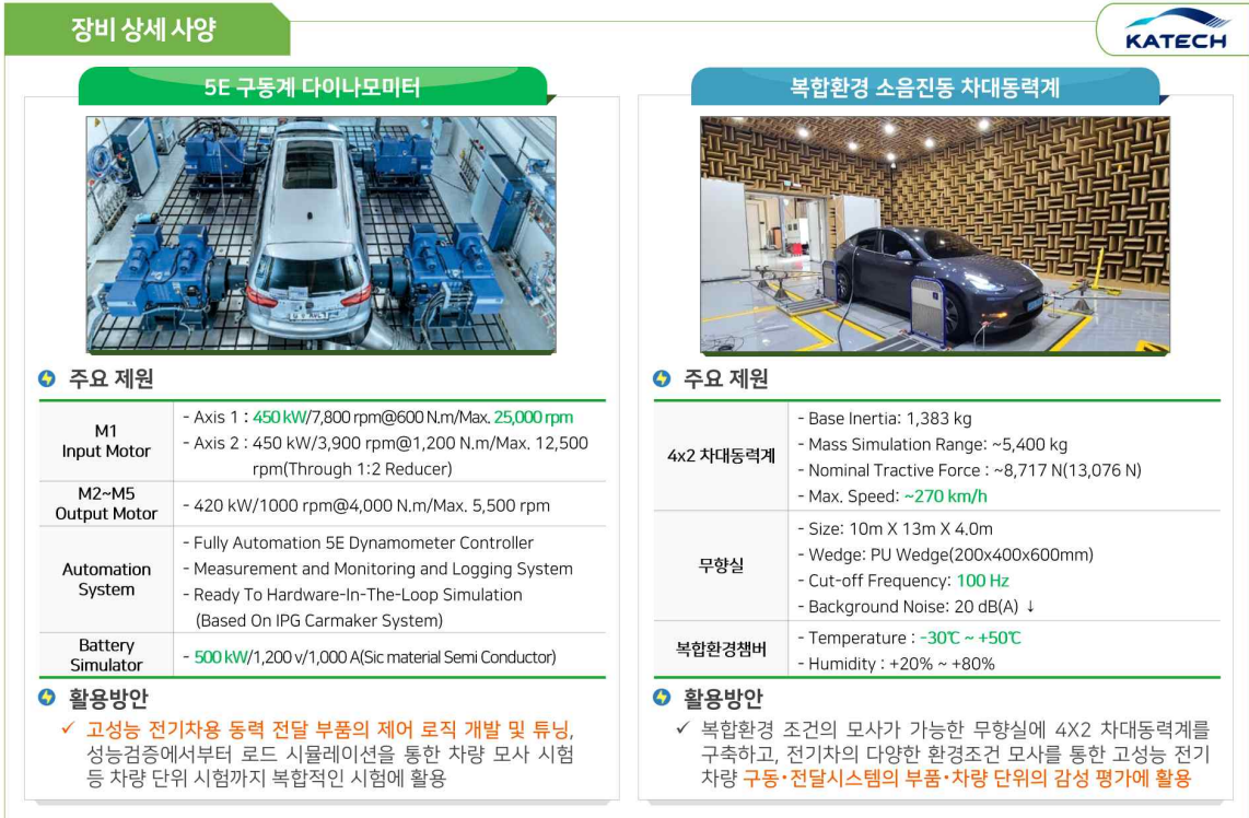
Fig. 1 Detailed Specifications of Equipment Introduced for the Construction Project
